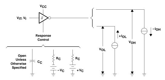
Figure 1. Receiver Section Test Circuit ( $V_{IT+}$ ,  $V_{IT-}$ ,  $V_{OH}$ ,  $V_{OL}$ )
