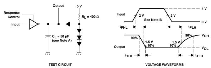
NOTES: A.  $C_L$  includes probe and jig capacitance.
